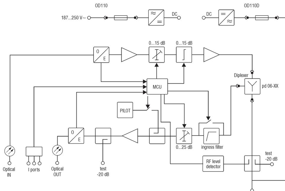
**Remotely monitored parameters of the nodes OD110, OD110D using monitoring subsystem "MasterWatch":**
