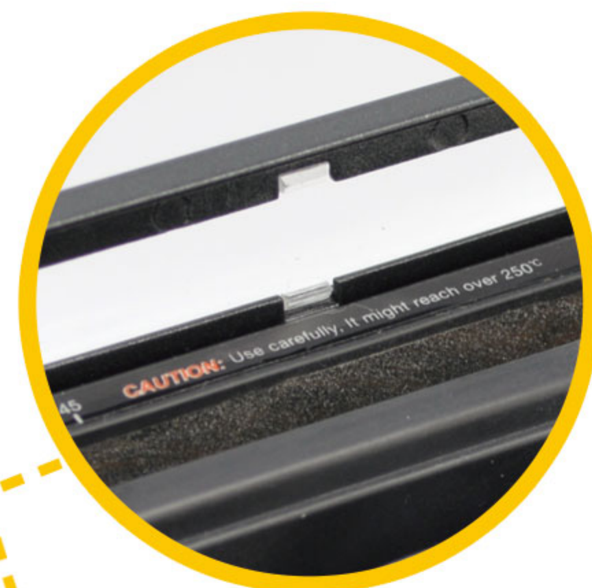
Heating Time - 18 sec <60mm sleeve>
