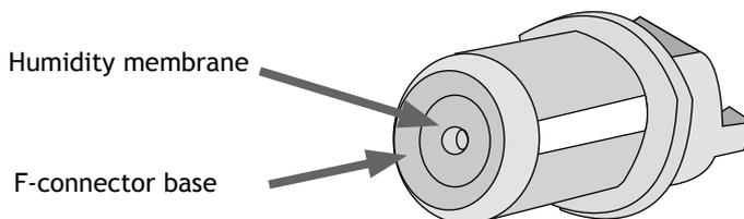
Based on these results it is concluded that the Signia housing it-self is IP class 64 (dust and dripping water tight). With cables and/or terminators mounted on all ports it is concluded that the Signia housing is IP class 67.
