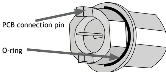
To ensure potential corrosion over a long period of time have no effect on the electrical performance, the outershield of the F-connector is soldered directly onto the printed circuit board (PCB).
