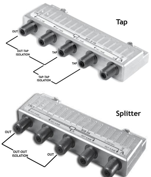
For isolation measurements a signal is applied to a connector and the output is measured on the other connectors.
